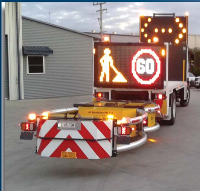
Traffic attenuator with variable roadwork signage
