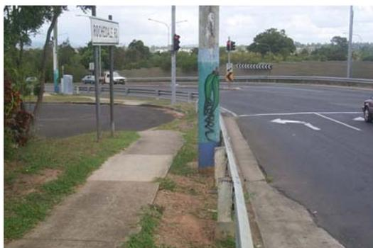
**Figure 8.116 It appears that the barrier is there to shield the pole but will not perform adequately in a crash**
