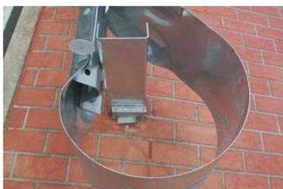
**Figure 8.95** Another view of slip base mechanism in Figure 8.94
