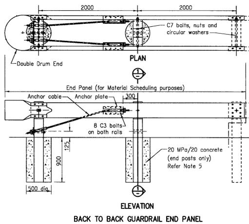
**Figure 8.106 BANNED** end treatment previously used for back-to-back guardrail installations
