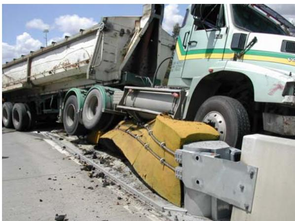
**Figure 8.87 Rubber crash cushion and 22,000kg articulated vehicle**
