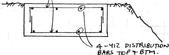
Figure 8.119 Footing assembly for culvert crossings Sheet 1 of 4 (refer also to Figure 8.117)
