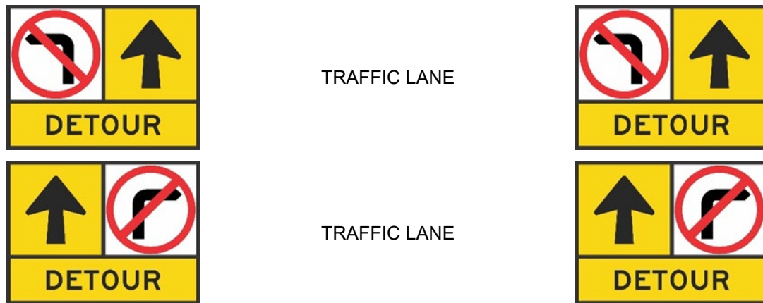
Figure 4.2.2(a) – Example multi-message signs with No Left / No Right Turn prohibition panels
