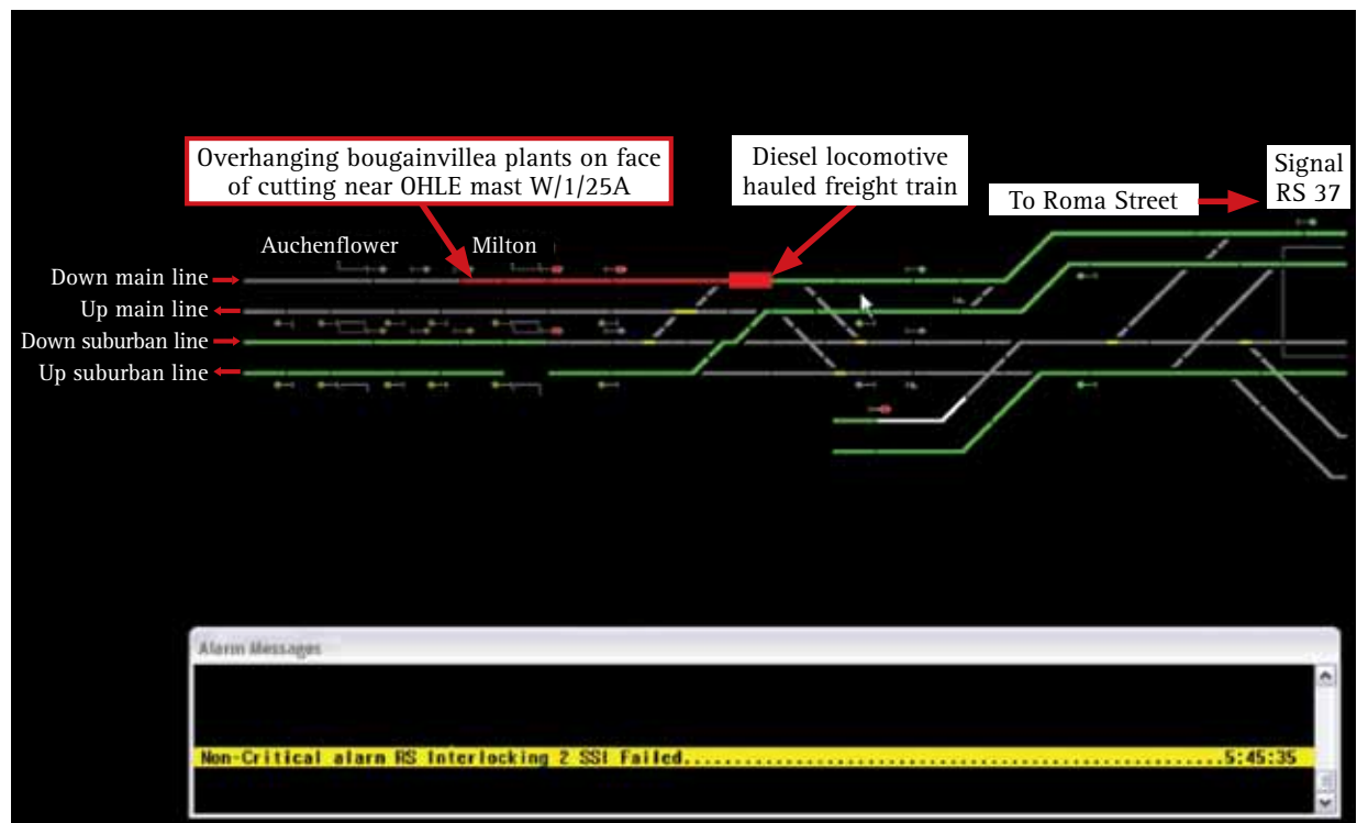
Figure 16 - Train Controller's screen at the time of signalling fault alarm (unrelated screen information removed).
